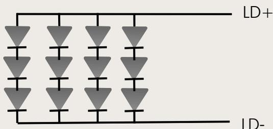
(Forward voltage of LEDs: 2.7 V to 3.4 V)
