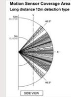
**McMS** is available as add\_on module for connecting to the main charge controller unit. It is available in different sense-ranges, from 6m to 15m. It comes with 3 way relimate connector to be directly plugged in the main unit which has 3-way base provided exclusively for this module.
