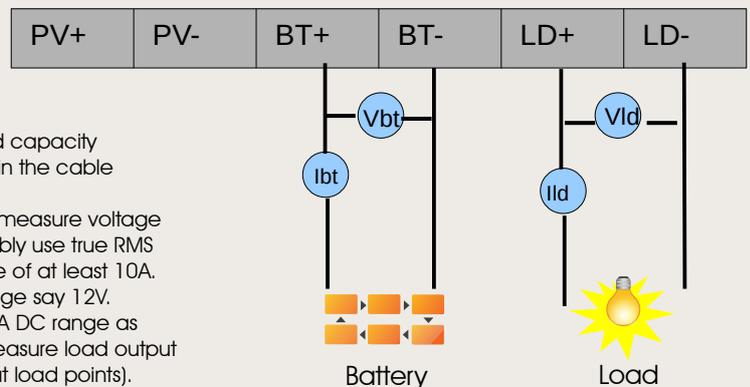
Precautions should be taken to use rated capacity wires to make connections so that drop in the cable is minimised.
