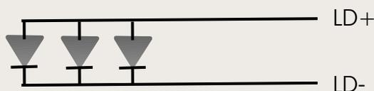
(Forward voltage of LEDs: 8.2V to 10 V)
